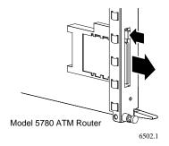
Remove the flash memory card by gently pulling the card away from the connectors, or by pressing the button next to the slot.
